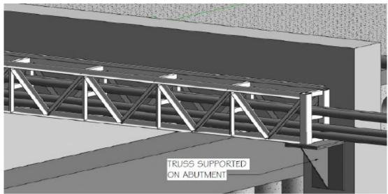
Figure 4.3 – Indicative image of cable trough
